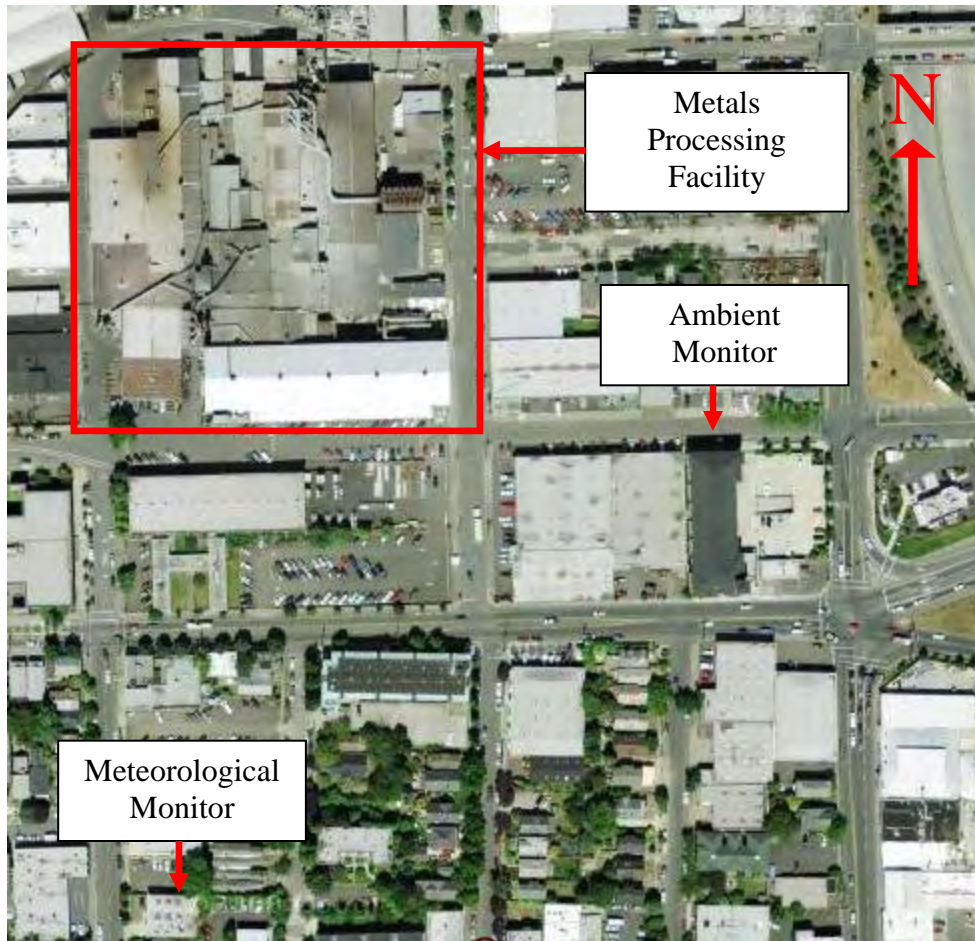
Figure 3. Aerial view of the relative location of the metals processing facility and the ambient and meteorological monitors.
