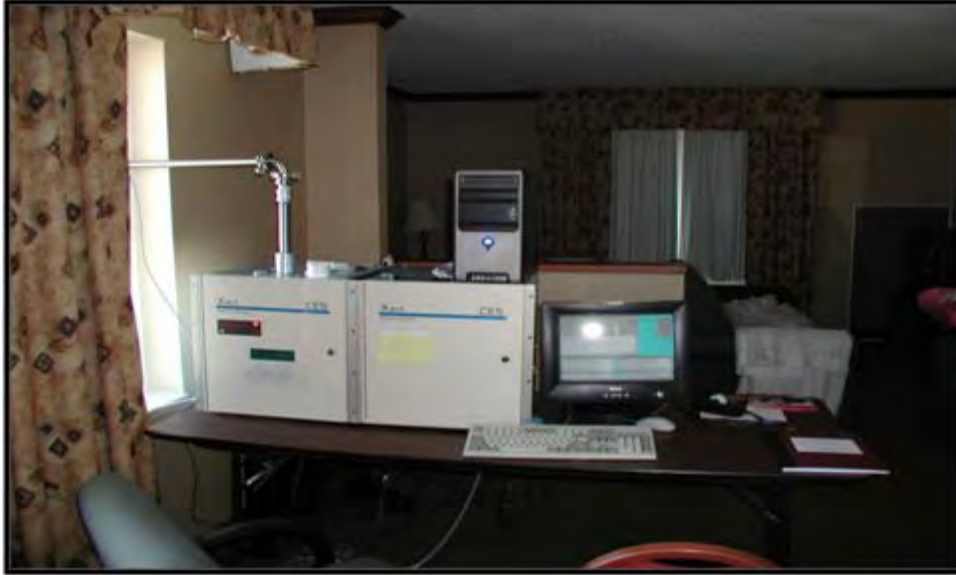
Figure 2. The Xact 620 experimental setup as deployed for this experiment.
